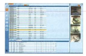
You can also select to group assets by a unique field, for example, pipe ID, then expand all rows to see which assets have multiple inspections. A user can then select an inspection to review the media in the right window.
