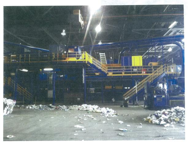
Single stream is made possible through the use of various mechanized screens and optical sorting technologies. Waste Management continues to advance in the area of single-stream recycling, with efforts to make these programs easy and cost effective.
