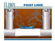
Using our proprietary LFS Point Liner, LiquiForce can repair isolated areas in diameters up to 24" without using disruptive and time consuming excavation methods. Utilizing time proven design principals as per ASTM F1216, we are able to install sectional CIPP liners at any
