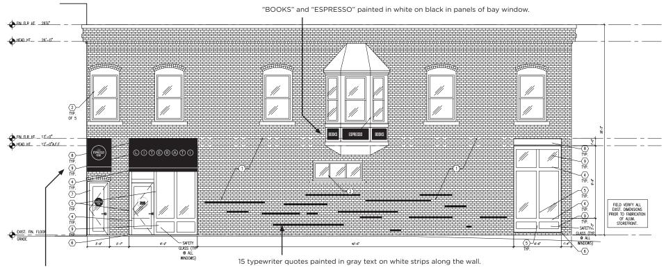
2 black awnings. 1 above each door on South Fourth Avenue. Awnings will be attached in joints between masonry units.
