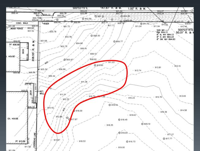
Water run off is perpendicular to the to the hill (assisted by gravity on the steeper gradients):
