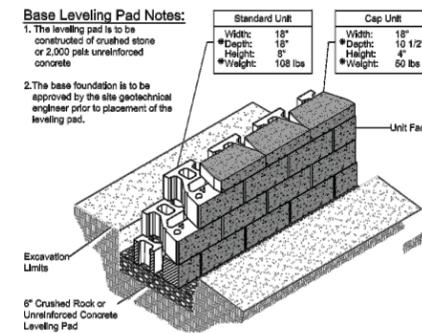
Standard Unit/Base Pad Isometric Section View
