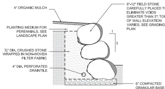
5 DRY-LAID STONE RETAINING WALL
