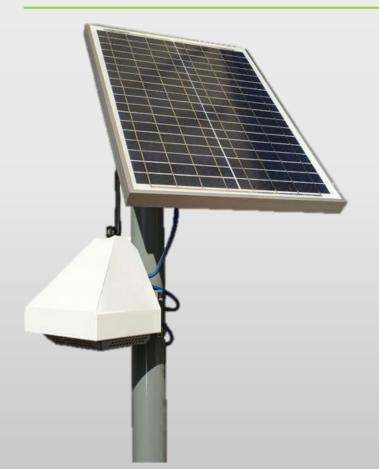
The City is installing solar-powered AQMesh sensor suites. These measure:
