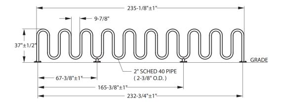
This rack claims to have a capacity for 21 bikes. Some very simple math would show, then, that it does not meet the city's existing standards, which again state: "One Bicycle Parking Space shall consist of a space not less than **two feet wide** by six feet long". In this rack, bicycle parking spaces are - interpreting measurements generously - about 1 foot wide, not 2.
