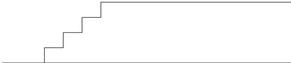
This is a normal staircase, with four 8" risers and 10" treads.
