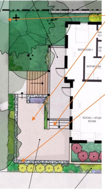
ORIGINAL DESIGN – STAIRS REQUESTED TO MOVE TOWARD HOUSE AND REMOVE HANDRAIL REDESIGNED LOWER ENTRY BASED ON HDC REQUEST GRADE FALLS ACROSS PROPERTY FRONTAGE, ELEVATION OF FRONT PATIO AREA IS THE SAME AS THE NORTH PROPERTY SIDEWALK
