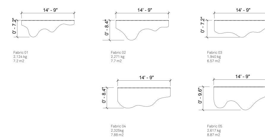
FABRIC PATTERN Weight of steel wire is not calculated-SITE 04 - A2 SUNSET SCALE: 1/8" = 1'-0"
