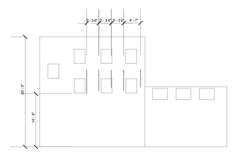
site 04 - a2 sunset goodyear building east building alleyway width - 16' - 2" brick dimensions - 8-1/8" x 2-1/2" mortar joint width: 1/2"
