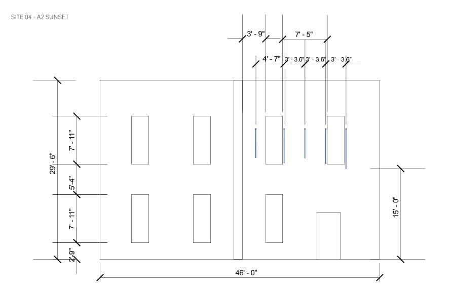
site 04 - a2 sunset cafe zola west building alleyway width - 16' - 2" brick dimensions - 7-5/8" x 2-5/8" mortar joint width: 3/8"
