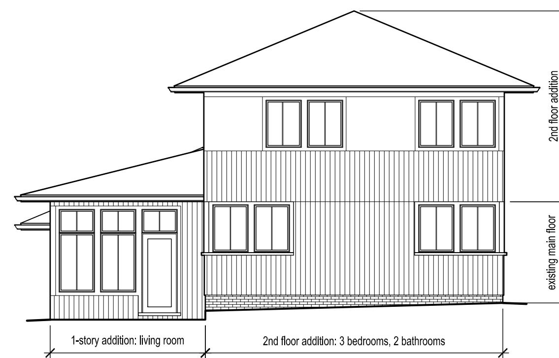
1 EAST ELEVATION - PROPOSED 1/8" = 1'-0"
