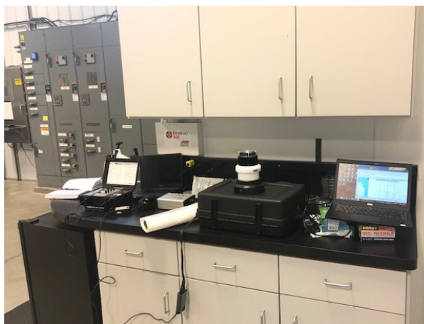
Right sizing the design of UV equipment relies on assessment of effluent water quality. Onsite portable testing (laboratory on left) can be performed to supplement available data. Collimated Beam testing can provide an efficient (time and cost) means to log removal and UV dosage (figure on right).
