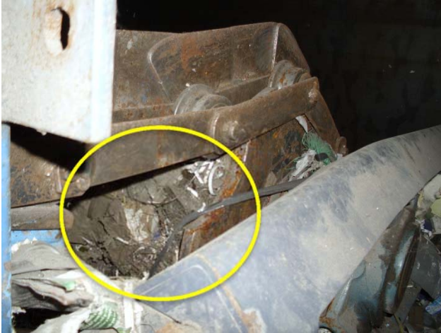
Shaft is wrapped inside of belt.
