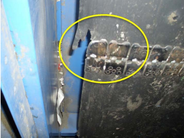
Belt is torn, laced improperly. Replacement recommended.
