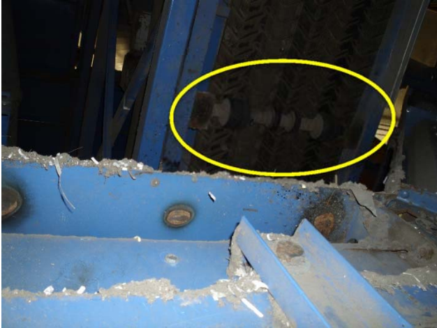
Return rollers are worn and need to be replaced.
