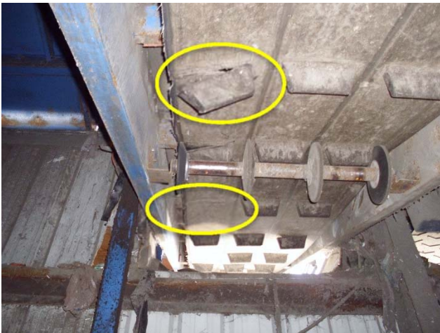
Belt need to be replaced. Cleats are torn/missing.
