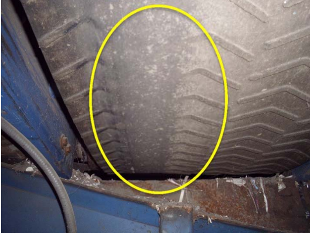
Belt is worn, replacement required.
