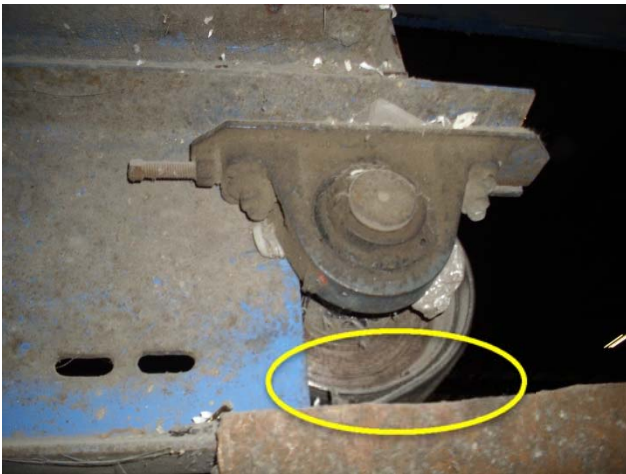
Return rollers are damaged. Replacement required.
