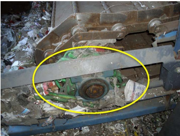
D hole bars are missing/broken.
