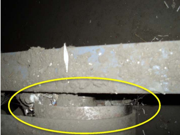
Picture shows a severely worn pulley and belt tracking veering off. Pulleys to be replaced.
