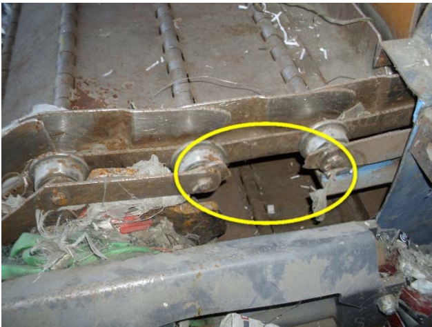
D hole bars are missing/broken.
