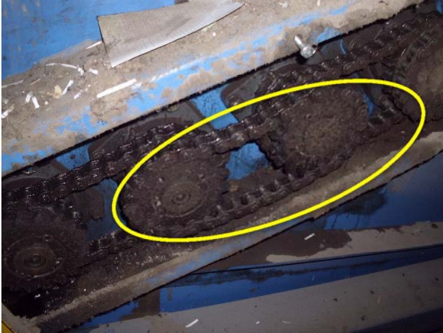
Chains are stretched and sprockets are worn, replacement required.
