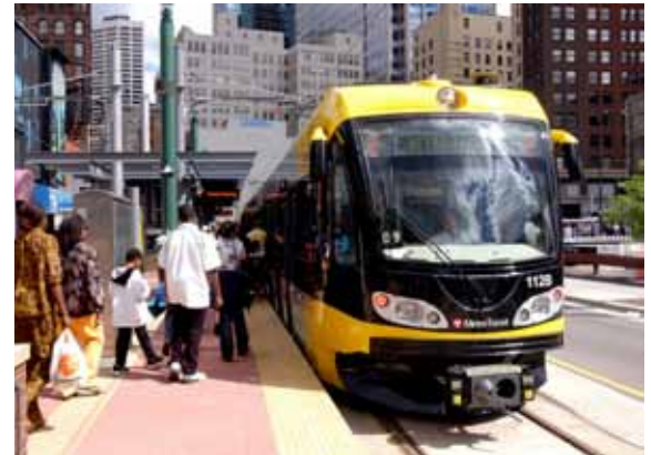
Stations and vehicles are fully ADA compliant with level boarding and four wheelchair locations per vehicle
