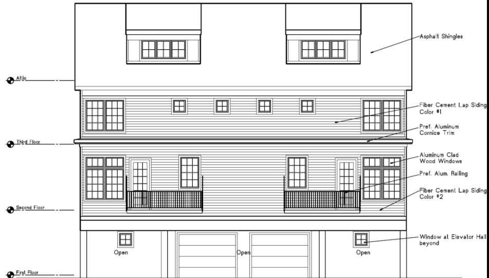
Rear (West) Elevation Fourth Ave. Building Scale: 1/4" = 1'-0"
