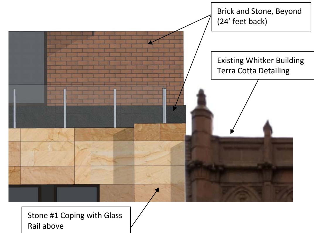
Enlarged View of Relation between 315 S. Main and Whitker Building Cornices (above)
