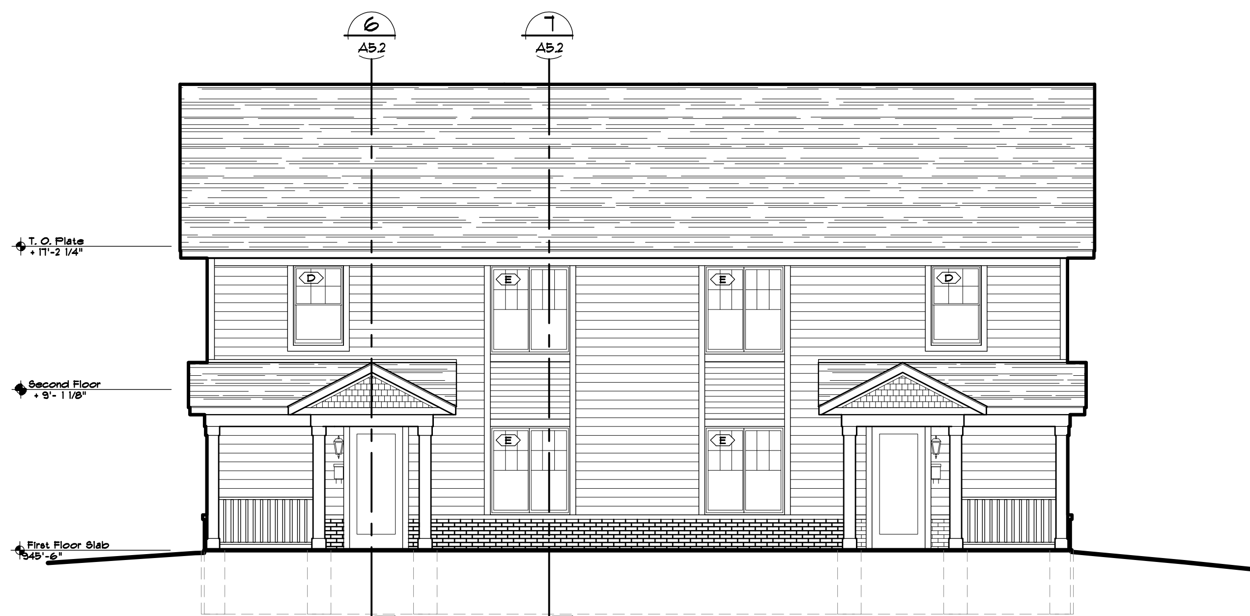
FRONT ELEVATION Platt East - Building B SCALE: 3/16"=1'-0"
