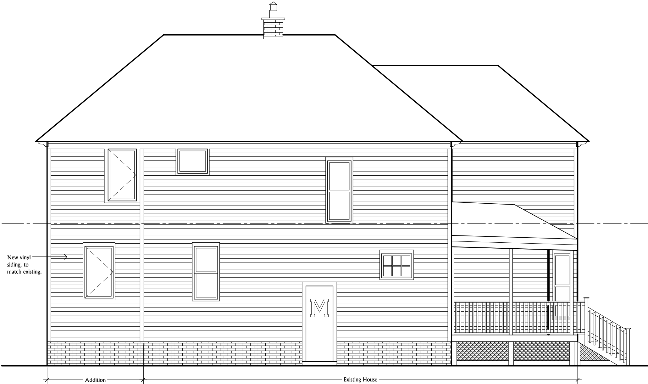
Proposed West Elevation - 601 E. Hoover Scale: \frac{3}{16}'' = 1'-0''
