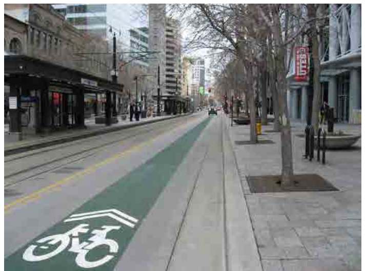
A “super sharrow” reinforcing the notion that a bike may use the full lane of the road.
