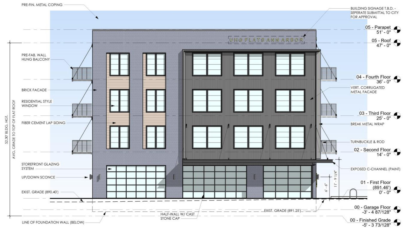
Front (East) Elevation
