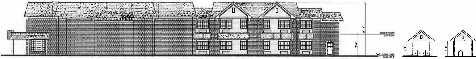
WEST ELEVATION - EXISTING RENOVATED SCALE: 1/8" = 1'-0"
