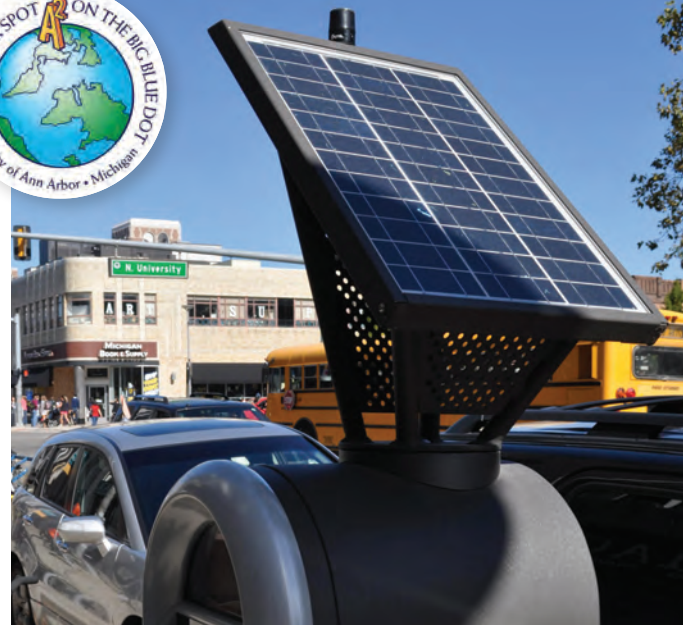
(above) A solar powered parking meter in downtown Ann Arbor. (left) Ann Arbor was the first city in the nation to convert its streetlights to LED.
