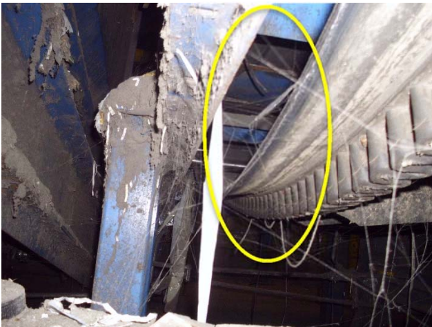
Belt tensioning is off, return rollers required to enhance optimal use.
