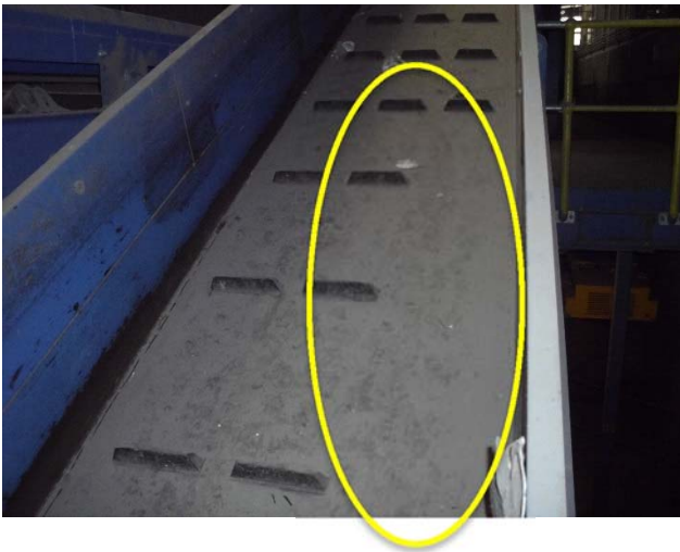
Belt is worn and need to be replaced. Missing cleats.
