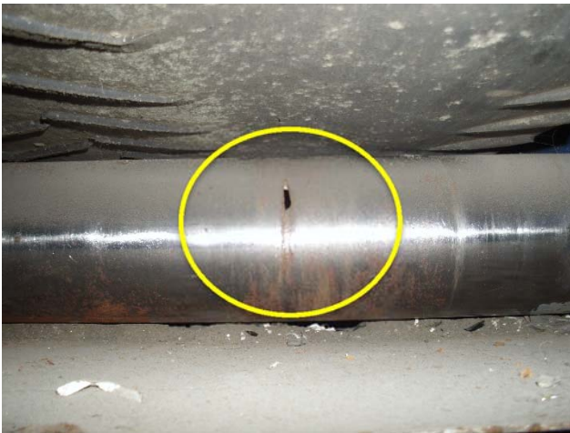
Return rollers are damaged. Replacement required.
