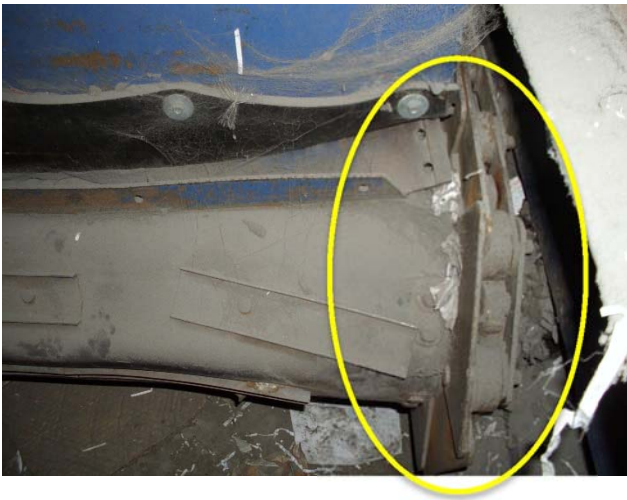
Belt is torn/worn, replacement required.
