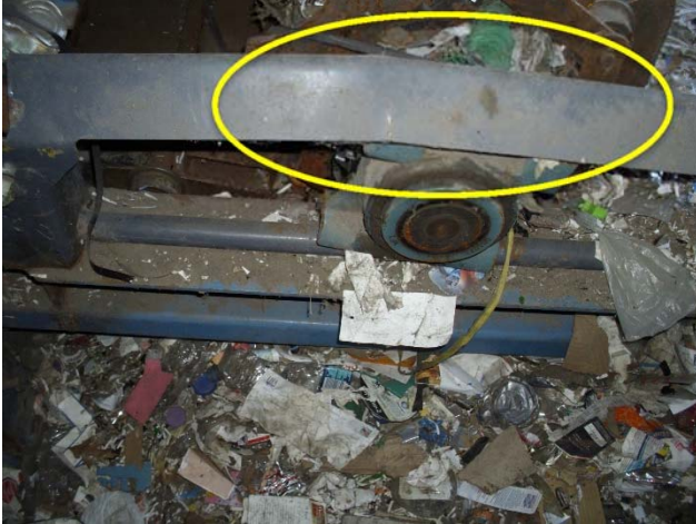
Take up is bent. Shaft is wrapped.
