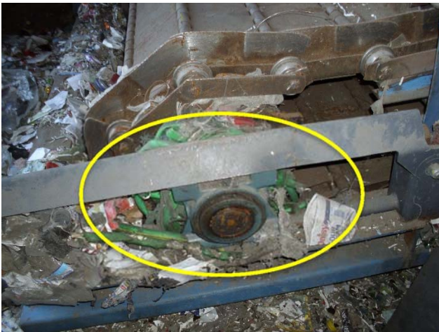
D hole bars are missing/broken.
