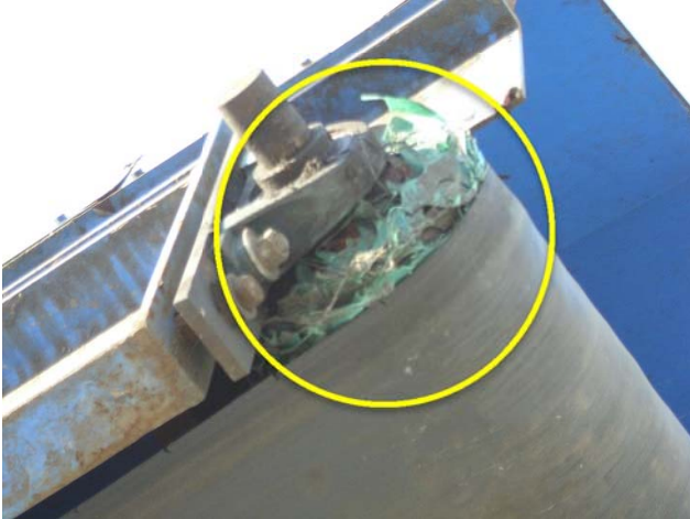
Pulley is wrapped.
