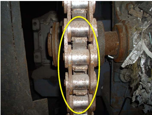
Head sprocket and Motor sprocket needs to be replaced. When sprockets are replaced, it is advised to change chain.
