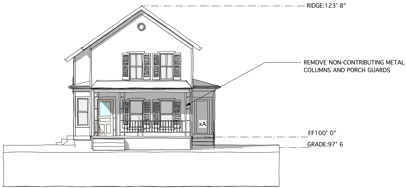
EXISTING EAST ELEVATION
