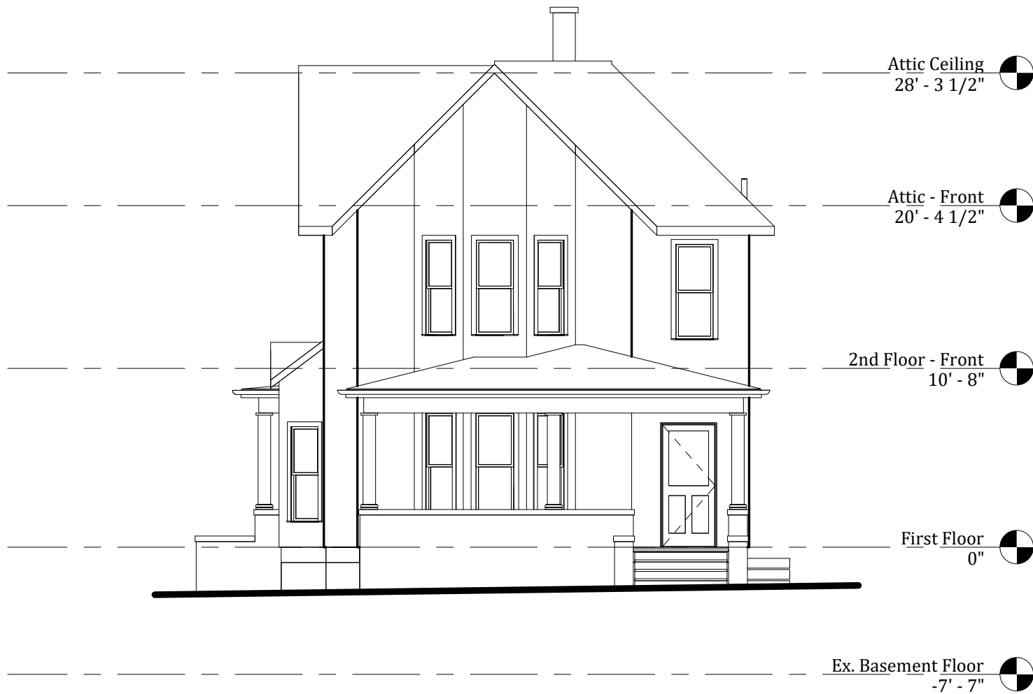
① Existing East Elevation 1/8" = 1'-0"
