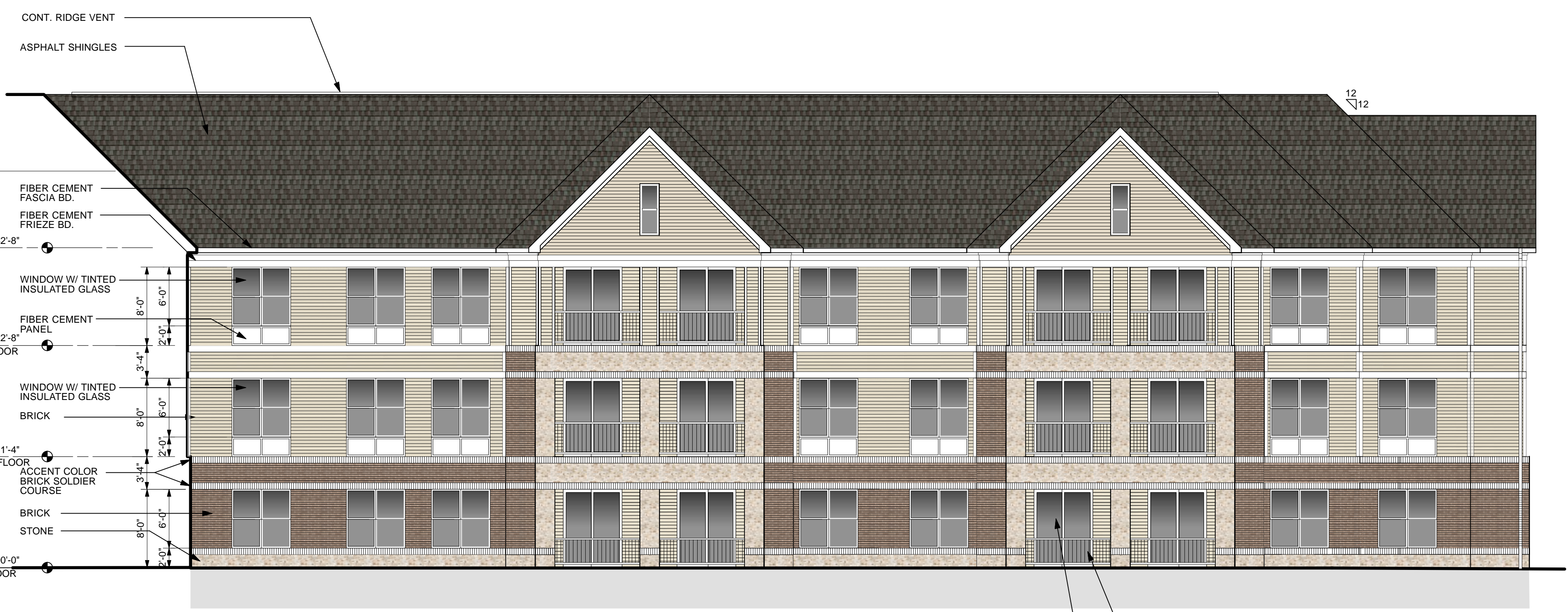
3 EAST ELEVATION A3.2 SCALE 1/8" = 1'-0"
