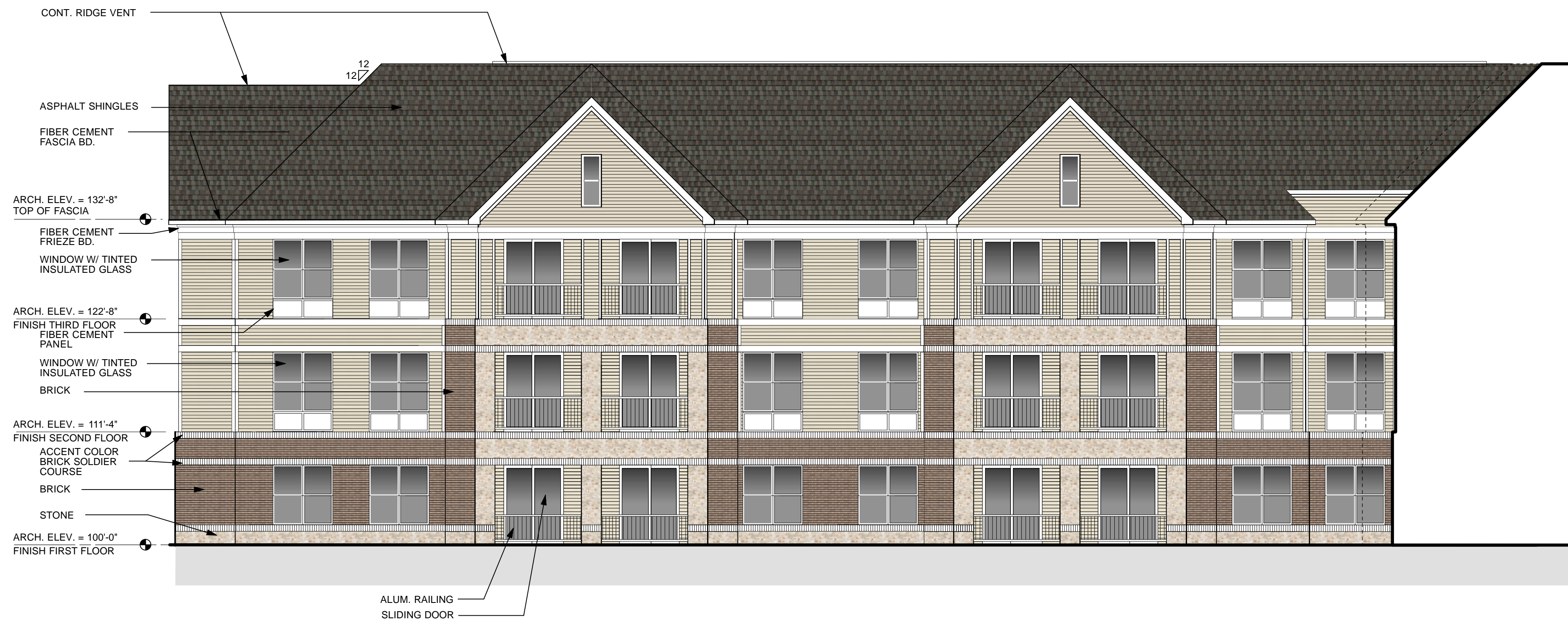
4 SOUTHEAST ELEVATION A3.1 SCALE 1/8" = 1'-0"
