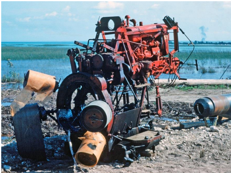
Photo E Trudgen Photo of Pipe Wrapping Machine 00010370012.tif
