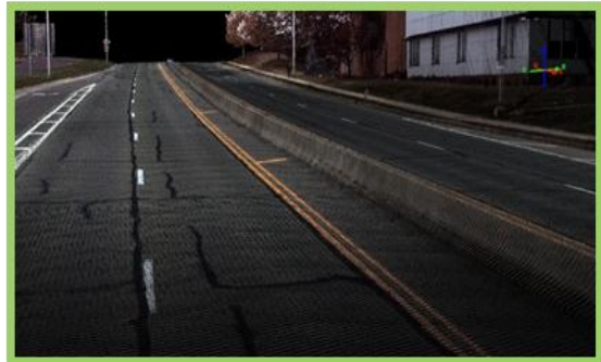
Snippet of point cloud data with real world color
