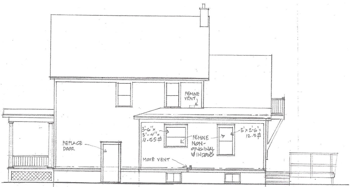
EXISTING SOUTH ELEVATION
