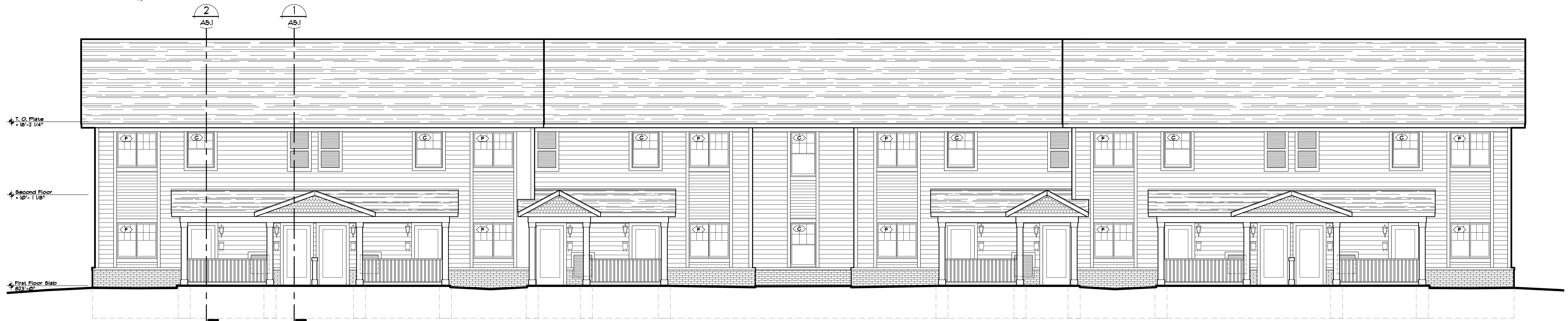
FRONT ELEVATION Platt East - Building F SCALE: 3/16"=1'-0"
