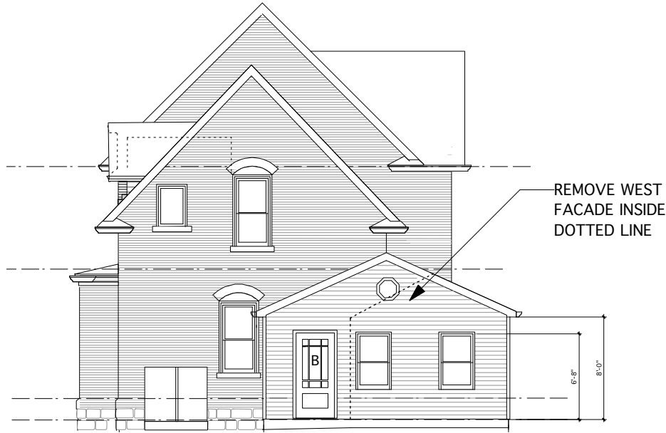
WEST ELEVATION EXISTING SCALE: 3/32" = 1'-0"
